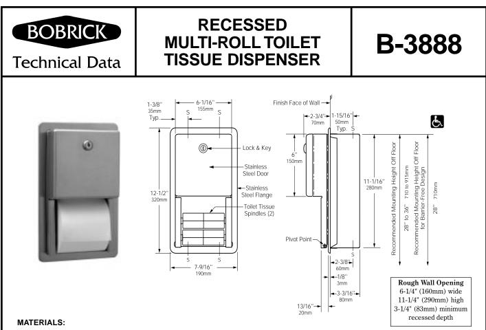
Cabinet — 18-8 S, type-304, 22-gauge (0.8mm) stainless steel. All-welded construction. Exposed surfaces have satin finish.
